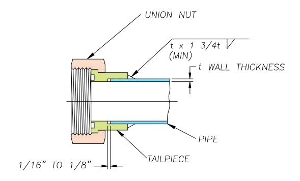
FITTINGS DESIGNED TO COMPLY WITH WELDING STANDARD MIL-STD-22D FOR PIPING CLASS P-1 AS SHOWN.
