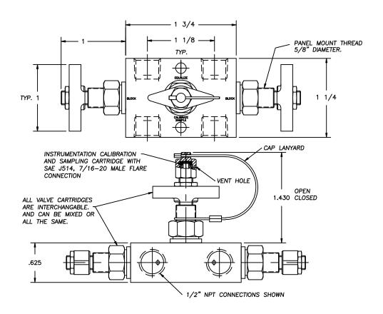
CAT M4300 INSTRUMENT VALVE MANIFOLD BLOCK, BLEED AND CALIBRATION
