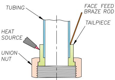
BRAZING IS A RELIABLE, ECONOMICAL HEAT SEALED JOINT. ALL METHODS OF BRAZING; TORCH, INDUCTION HEATING, FURNACE, PREINSERTED RING OR FACE FED CAN BE USED.
