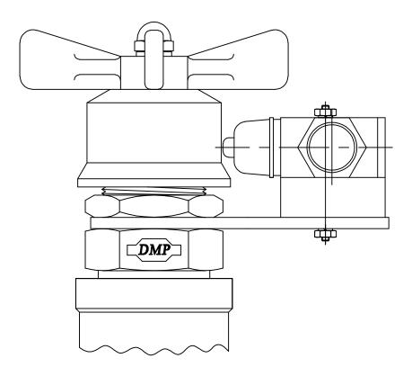
LIMIT SWITCHES (-LS) CAN BE FURNISHED WITH ANY FFS VALVE OR CARTRIDGE. SWITCHES AVAILABLE: SINGLE POLE DOUBLE THROW.
