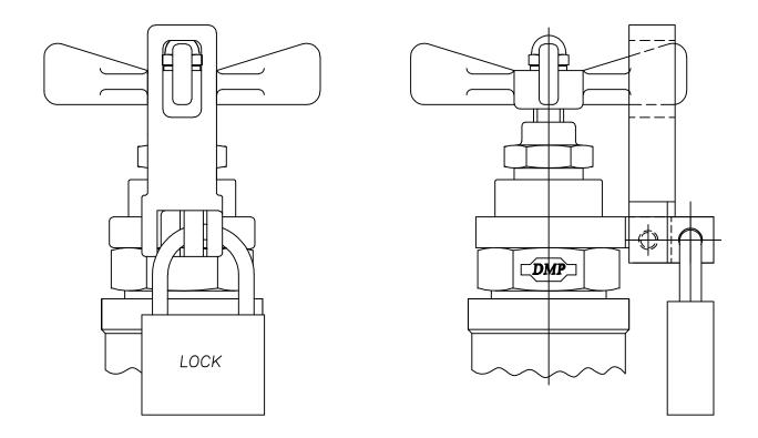
THE LOCKING DEVICE M3, SHOWN ABOVE IS AVAILABLE FOR ANY HAND OPERATED VALVE TO PREVENT ACCIDENTAL TURNING OF THE HANDLE. THE SHACKLE, ALIGNED WITH ON OF THE HANDLE SPOKES, CAN BE LOCKED IN PLACE BY USE OF A PADLOCK (NOT SUPPLIED WITH DEVICE).
