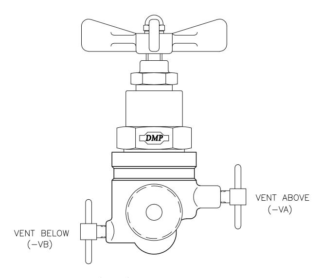
VENT (VA OR VB) FFS VALVES CAN BE FURNISHED WITH PROVISION FOR VENTING ABOVE THE SEAT (-VA) OR BELOW THE SEAT (-VB). THIS PROVISION IS DESIRABLE FOR VENTING (BLEEDING) AIR THAT MIGHT FORM POCKETS IN A HYDRAULIC SYSTEM OR FOR TAKING SAMPLES OF SYSTEM FLUID. NOTE: BECAUSE OF THEIR CONFIGURATION, ANGLE VALVES ARE LIMITED TO ONLY VENTING ABOVE THE SEAT (-VA).
